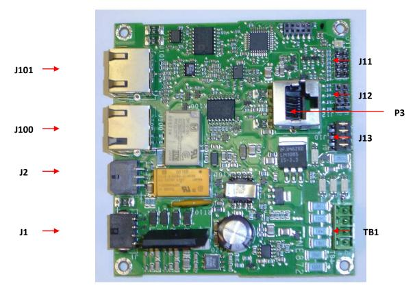
Figure 17: NE872A Remote Distribution Module
