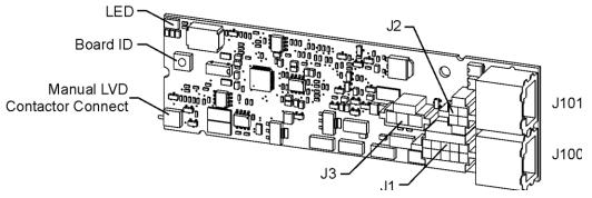
Figure 25 QS871A Remote Distribution Module
