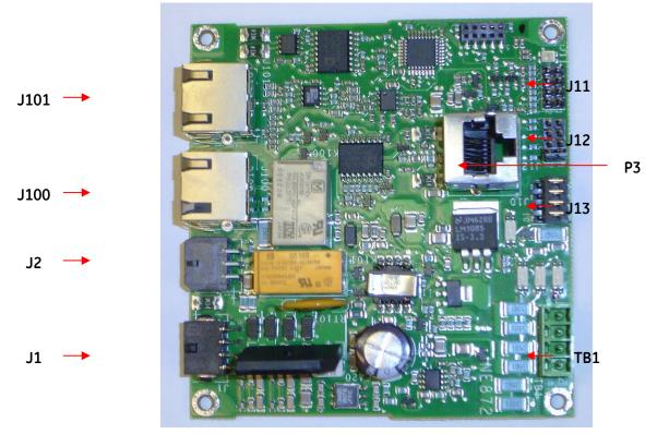
Figure 22 NE872A Remote Distribution Module
