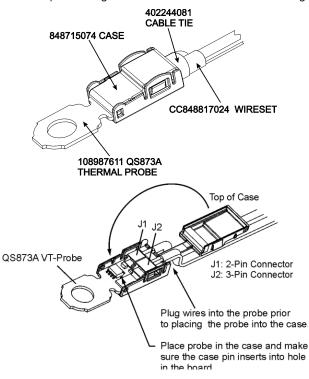
Figure 17 QS873A Voltage/Thermal Probe (VT-Probe)
