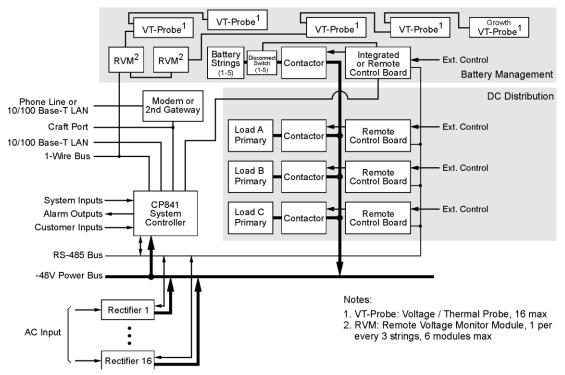
Figure 6 General Power System Block Diagram
