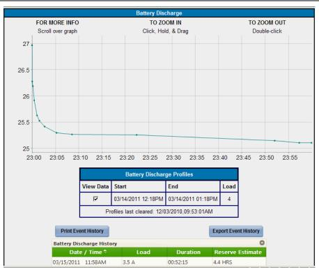
The Battery Discharge History events provide date and time, average load during discharge, and duration of each recorded battery discharge event. The reserve time will be provided if available for each event. Selecting a color from the view data screen will allow the discharge curve profiles to be graphed and overlayed.
