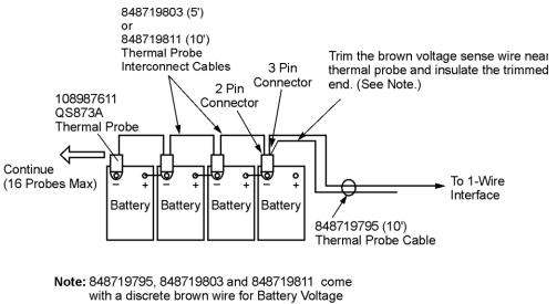
with a discrete brown wire for Battery Voltage Sense. When ES771A Modules are NOT used, trim and insulate this wire
