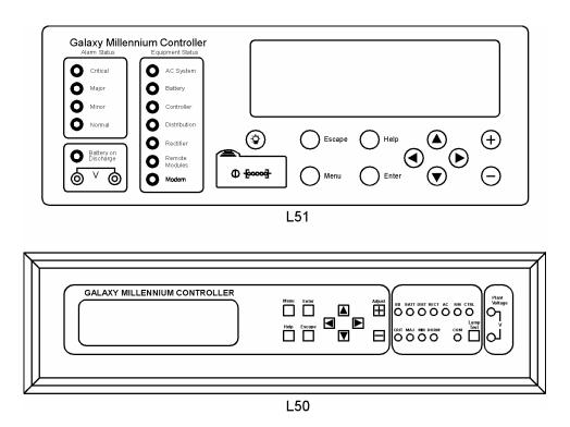
Figure 4-5: Controller Front Panel Displays
