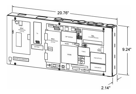
Figure 2-1: Controller Dimensions
