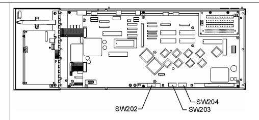
Figure 6-7: Millennium Controller Switch Locations
