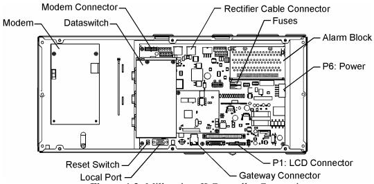
Figure 4-3: Millennium II Controller Connections
