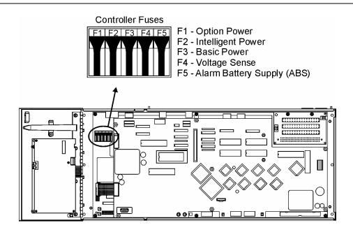
Figure 6-4: Millennium Controller Fuse Positions
