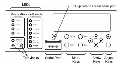
Figure 4-6: Detailed Controller Front Panel Display – L51/52
