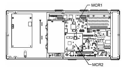
Figure 2-3: MCR1 and MCR2 Boards
