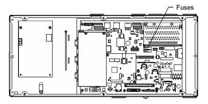
Figure 4-4: Millennium Controller Fuses
