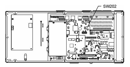
Figure 4-7: Millennium II Controller Dip Switches
