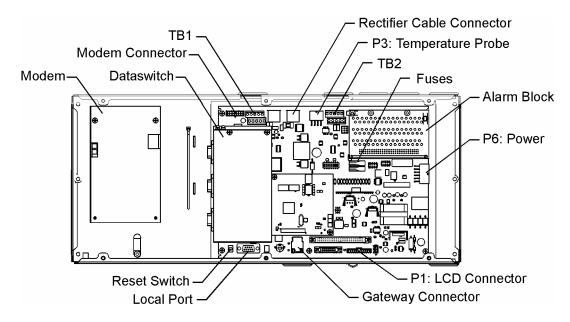
Figure 4-2: Millennium II Controller Connections
