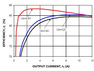
Figure 13. Converter Efficiency versus output current.
