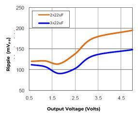
Figure 37. Input ripple voltage for various output voltages with  $2x22 \ \mu F$  or  $3x22 \ \mu F$  ceramic capacitors at the input (12A load). Input voltage is 12V.
