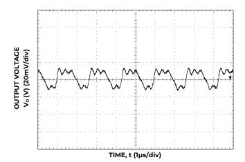
Figure 15. Typical output ripple and noise (C₀=22µF ceramic, V<sub>IN</sub> = 12V, I₀ = I₀,max,).
