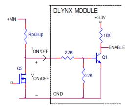
Figure 40. Circuit configuration for using negative On/Off logic. Monotonic Start-up and Shutdown
