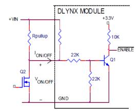
Figure 39. Circuit configuration for using positive On/Off logic.
