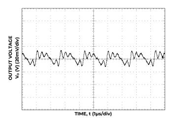
Figure 3. Typical output ripple and noise  $(C_0=22\mu F \text{ ceramic}, V_{IN}=12V, I_0=I_{0,max}).$
