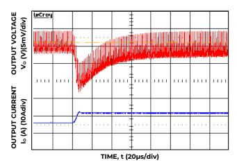
Figure 4. Transient Response to Dynamic Load Change from 50% to 100% at 12V<sub>in</sub>, C<sub>out</sub>=3x47µF+6x330µF, C<sub>Tune</sub>=47nF, R<sub>Tune</sub>=180ohm.
