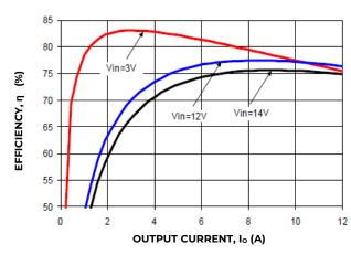
Figure 1. Converter Efficiency versus output current.
