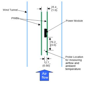
Figure 49. Thermal Test Setup.
