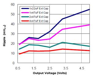
Figure 38. Output ripple voltage for various output voltages with external 1x22  $\mu$ F, 1x47  $\mu$ F, or 4x47  $\mu$ F ceramic capacitors at the output (12A load). Input voltage is 12V.
