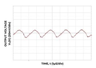
Figure 27. Typical output ripple ( $C_0$ =7x22 $\mu$ F ceramic,  $V_{IN}$  = 12V, Io =  $I_{o,max,}$ ).
