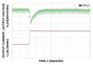
Figure 16. Transient Response to Dynamic Load Change from 50% to 100% at 12Vin, Cout= 7x47µF+2x330µF CTune=3900pF, RTune=300
