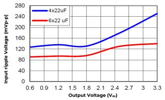
Figure 31. Input ripple voltage for various output voltages with 4x22 µF or 6x22 µF ceramic capacitors at the input (20A load).
