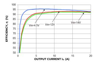
Figure 19. Converter Efficiency versus Output Current.
