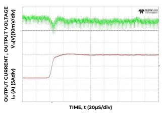
Figure 4. Transient Response to Dynamic Load Change from 50% to 100% at 12Vin, Cout= 7x47µF+9x330µF CTune=15nF, RTune=300
