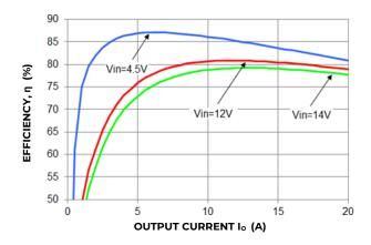
Figure 1. Converter Efficiency versus Output Current.
