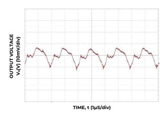
Figure 15. Typical output ripple ( $C_0$ =7x22 $\mu$ F ceramic,  $V_{IN}$  = 12V, Io =  $I_{o,max,}$ ).
