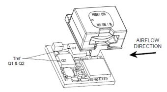
Figure 43. Preferred airflow direction and location of hotspot of the module (T<sub>ref</sub>).
