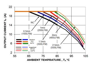
Figure 8 Derating Output Current versus
