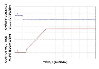
Figure 17. Typical Start-up Using On/Off Voltage (Io = I<sub>o,max</sub>).
