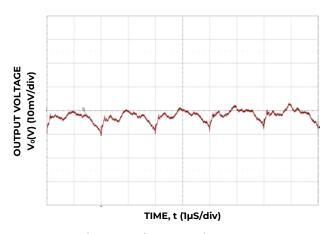
Figure 3. Typical output ripple ( $C_0=7x22\mu F$  ceramic,  $V_{IN}=12V$ ,  $Io=I_{o,max,}$ ).
