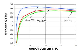
Figure 7. Converter Efficiency versus Output Current.
