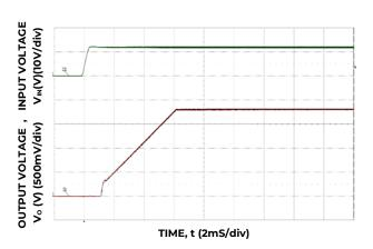
Figure 18. Typical Start-up Using Input Voltage ( $V_{IN} = 12V$ ,  $I_{O,max}$ ).
