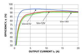
Figure 13. Converter Efficiency versus Output Current.
