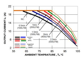
Figure 14. Derating Output Current versus
