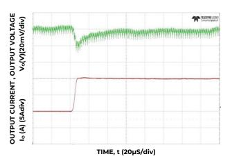
Figure 10. Transient Response to Dynamic Load Change from 50% to 100% at 12Vin, Cout= 7x47µF+4x330µF CTune=6800pF, RTune=300
