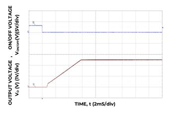
Figure 23. Typical Start-up Using On/Off Voltage (Io = I<sub>o,max</sub>).
