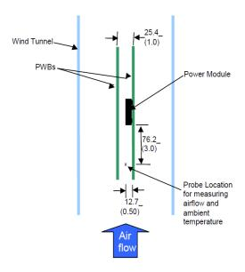
Figure 42. Thermal Test Setup.
