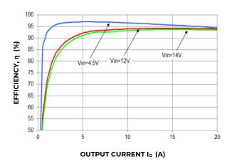
Figure 25. Converter Efficiency versus Output Current.
