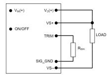
Figure 36. Circuit configuration for programming output voltage using an external resistor.
