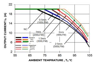
Figure 2. Derating Output Current versus Ambient
