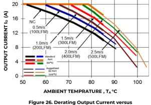
Figure 26. Derating Output Current versus
