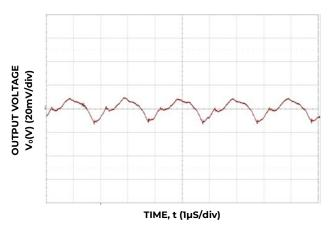
Figure 21. Typical output ripple ( $C_0=7x22\mu F$  ceramic,  $V_{IN}=12V$ ,  $Io=I_{O,max}$ ,).
