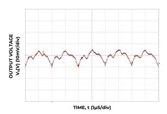
Figure 9. Typical output ripple ( $C_0=7x22\mu F$  ceramic,  $V_{IN}=12V$ ,  $Io=I_{o,max}$ ,).
