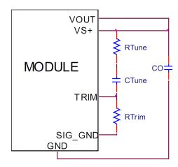
Figure. 40. Circuit diagram showing connection of RTUME and CTUNE to tune the control loop of the module.
