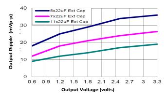
Figure 32. Output ripple voltage for various output voltages with external  $5x22 \mu F$ ,  $7x22 \mu F$  or  $11x22 \mu F$  ceramic capacitors at the output (20A load). Input voltage is 12V.
