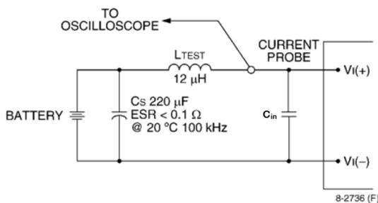
Note: Measure input reflected-ripple current with a simulated source inductance (LTEST) of 12 μH. Capacitor CS offsets possible battery impedance. Measure current as shown above.
