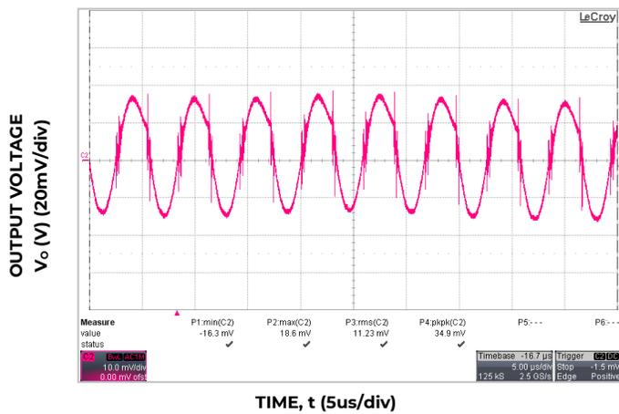
Figure 3. Typical output ripple and noise (C<sub>o</sub> = 650µF Ceramic + 650µF PosCap Oscon, V<sub>in</sub> = 54V, I<sub>o</sub> = I<sub>o,max</sub>).
