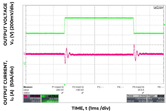
Figure 4. Dynamic Load Response, di/dt=1A/us; V<sub>in</sub>=V<sub>in,nom</sub>; T<sub>A</sub>=25°C; Load Change from I<sub>o</sub> = 50% to 75% of I<sub>o,max</sub>; C<sub>o</sub>=6160µF Ceramic;
