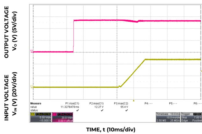
Figure 6. Typical Start-up Using Input Voltage (V<sub>in</sub> = 54V, I<sub>o</sub> = I<sub>o,max</sub>).
