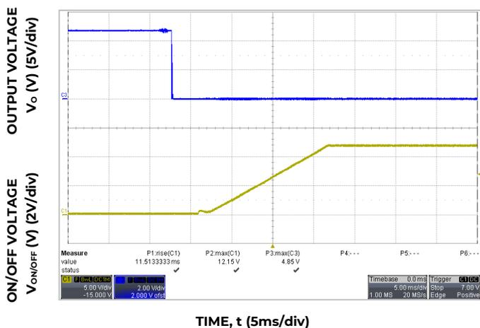
Figure 5. Typical Start-up Using On/Off Voltage (I<sub>o</sub> = I<sub>o,max</sub>).
