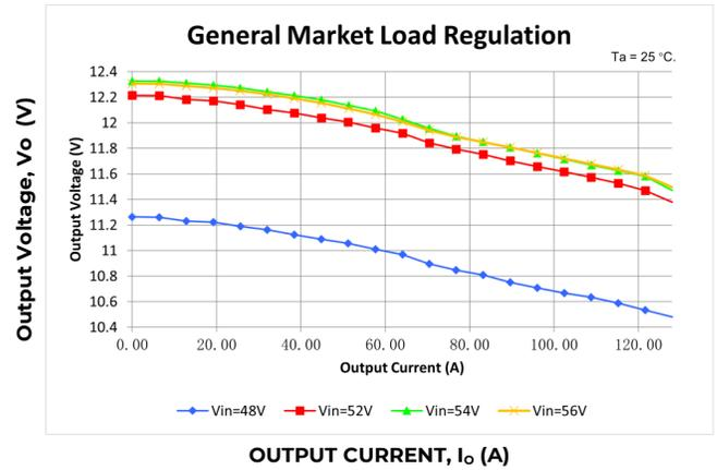
Figure 8. Typical Output Voltage Regulation vs Output Current
