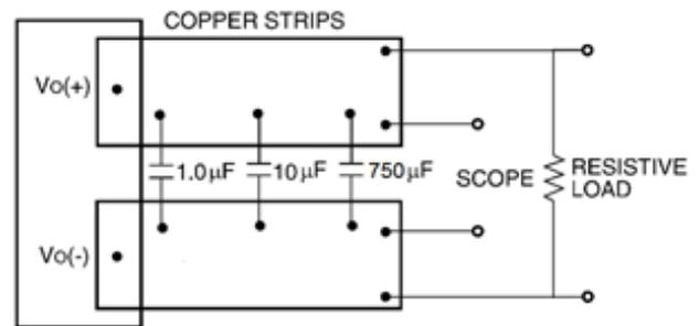
Note: Use a 1.0 μF ceramic capacitor, a 10 μF aluminum or tantalum capacitor and a 750 polymer capacitor. Scope measurement should be made using a BNC socket. Position the load between 51 mm and 76 mm (2 in. and 3 in.) from the module.
