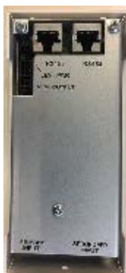
Figure 27 VIM1EC Meter RS485 Connection
