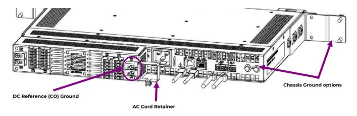
Step 4 - Connect DC Output and Battery, and DC Reference (CO) Ground
